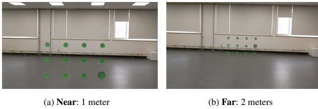
Figure 3: The experimental setup for both the ‘Near’(a) and ‘Far’(b) settings are depicted in these images, which were captured from the device. These images are representative of the device’s specified field of view (FOV) of 64.69°, as detailed in its technical documentation.
