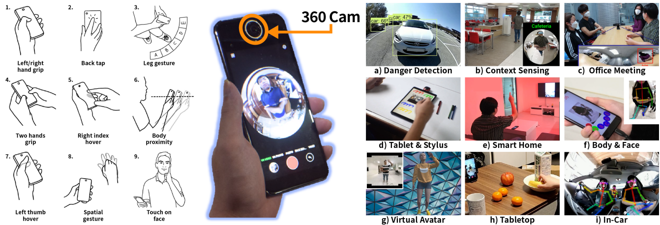
Figure 1: A mobile device with an omni-directional camera can capture a wide range of information about the user, including user's hand, body, and the surroundings. This allows various sensing techniques, which enable novel applications for mobile interaction, including danger detection while on the move, body pose for virtual avatar, spatial gestures for gaming, and more.
